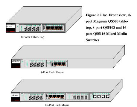
. Mixed-media combination modules (4-port modules with three fiber ports and one twisted-pair port) are supported in all of the Quad-Series Fiber Switch models. All quad-module manual-selection switches and LED's are located on the front panel, with the IEC standard AC power connector (and a manual ON - OFF power switch) located at the rear. Fan-driven cooling air flows left to right.
